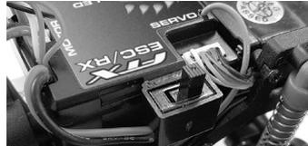
The ESC/receiver switch is located under the bodyshell of the model. Switch on the ESC/receiver switch shown here.
